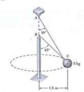
Two wires AC and BC are tied at C to a sphere which revolves at a constant speed v in the horizontal circle shown. Determine the range of values of v for which both wires remain taut.
