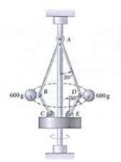
The 600 g flyballs of a centrifugal governor revolve at a constant speed v in the horizontal circle of 150 mm radius shown. Neglecting the weights of links AB, BC, AD, and DE and requiring that the links support only tensile forces, determine the range of the allowable values of v so that the magnitudes of the forces in the links do not exceed 80 N.
